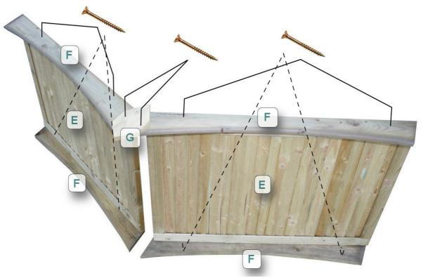
6. Fit fascia boards `F` to roof panels `E` using 8 x fixings `1`. Join roof panels `E` together with fascia cap `G` using 4 x fixings `3`.
